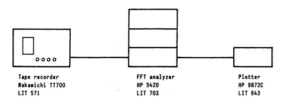
The signal was led from the taperecorder to the Fast Fourier Analyzer. This analyzer performs a narrow band, constant band width, frequency analysis.
